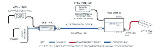
LONGSPAN Lite provides a full bandwidth link to a LONGSPAN Max Camera, locally
